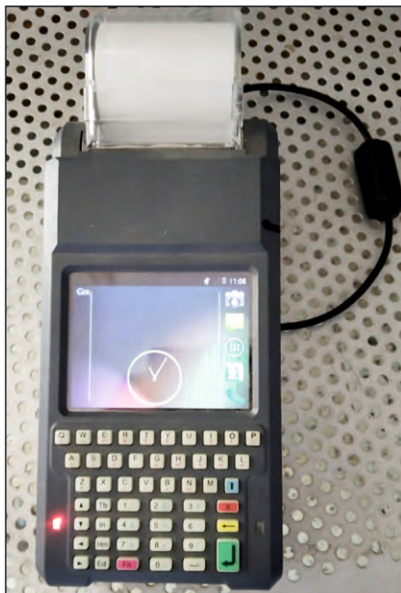
Handhold device used to integrate weighing machine through Bluetooth & Wifi
